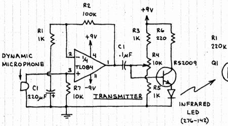
POINT THE LED AT QI AND ADJUST R4 UNTIL BEST VOICE QUALITY IS OBTAINED. (R4 APPLIES PREBIAS TO LED.) R6 LIMITS MAXIMUM LED CURRENT TO A SAFE 40 m A. USE RADIO SHACK 276-130
